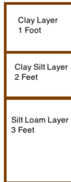
Figure 1: Example Soil Profile with Texture and Depth
